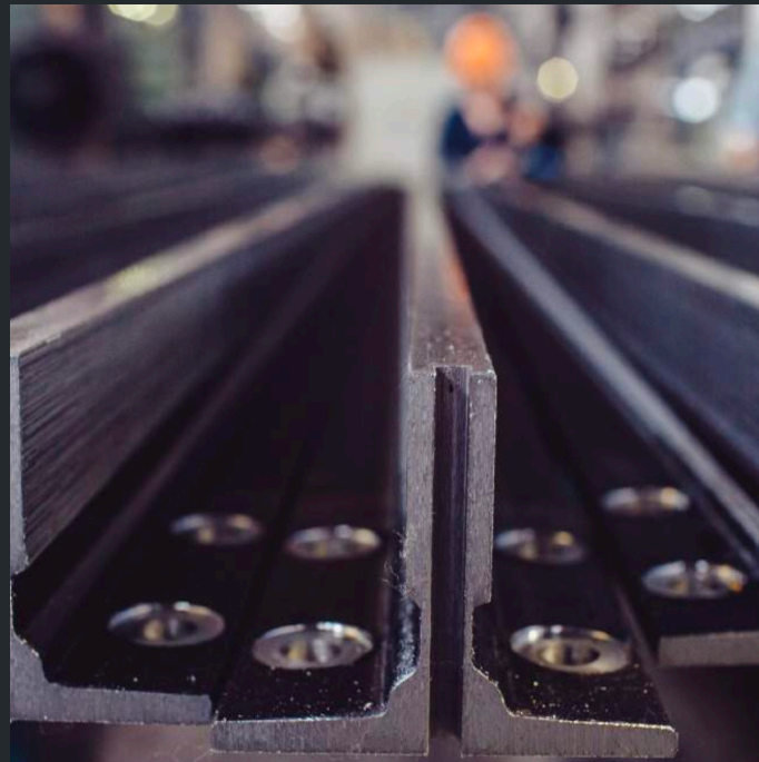
ELEVATOR GUIDE RAILS
